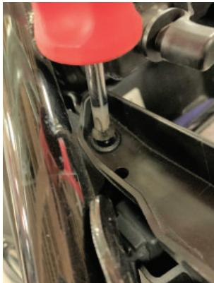
2. Remove stock panel by pushing towards back of motorcycle, while pulling outward.
