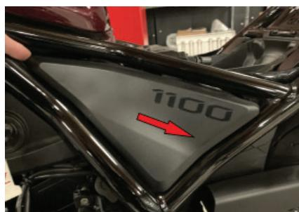
3. Install new side cover and mount using the supplied M5 Button Head Screw. Apply medium strength thread locking compound and torque to 26 in-lbs.
